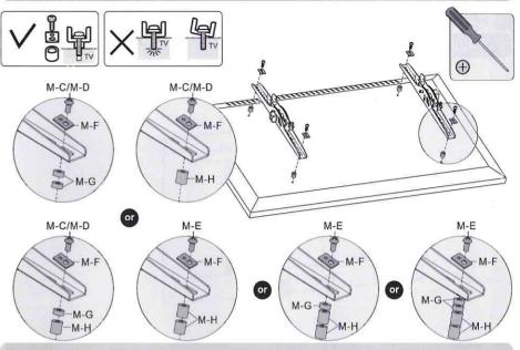
Note: Choose the appropriate screws, washers and spacers (if necessary) according to the type of screens.
